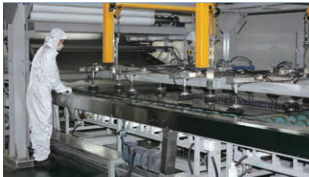
夹胶玻璃无尘合片室 Clean Room For Laminated Glass
