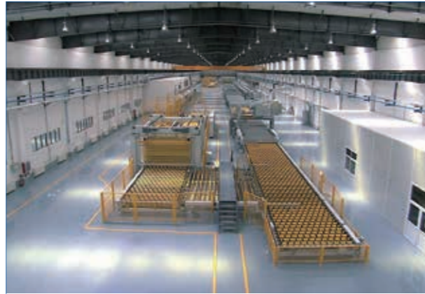
德国莱宝光学Low-E镀膜生产线 (年产能1000万平方米) Most advanced Low-E coating line of Leybold Germany (Annual capacity of 10 million square meters)
